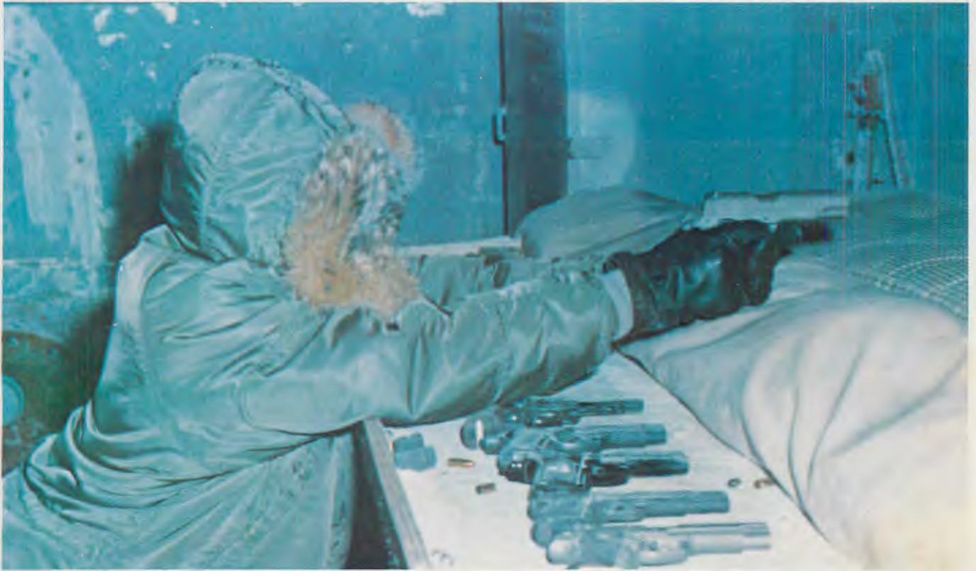
ABOVE: Test pistols must function in cold room's minus 60 degrees F. This hurdle alone eliminated some contenders. BELOW: Test pistols undergo mud bath in cement mixer. Afterwards they must shoot (minor manual assistance is allowed).
